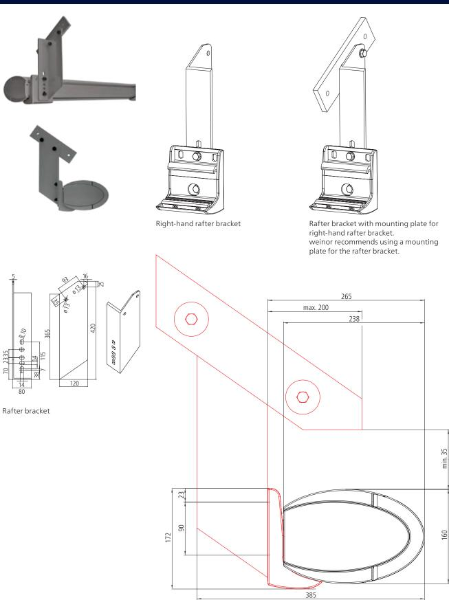
Side view: rafter bracket installation
